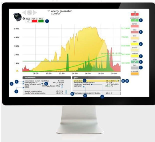
Figure 20 - Affichage Supervision Solar Log
